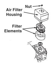
3. Check Air Filter (75) (See illustration above, right). Unscrew Air Filter Housing Nut and remove the Air Filter Housing and Filter Elements. If dirty or dusty, clean (refer to the Maintenance Section).
